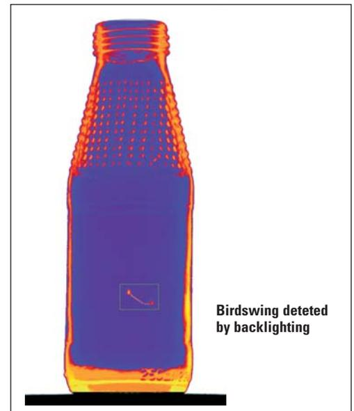
The best inspection is done by backlighting. Other methods relying on Near Infra Red radiation exists, but the results are not reliable. NIR reflections from neighbouring containers, difference in cooling and many other factors disturb the picture and the results are prone to misinterpretations. Therefore, the best way is to use backlighting where all NIR radiation is eliminated and a dependable illumination is arranged.
