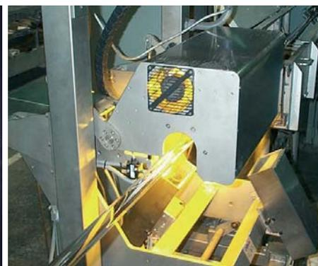
Tube inspection using powerful light. The system is installed at the line where the glass tubing is drawn at high speeds.
