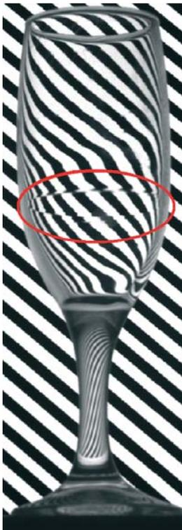
Mould ring enhanced by structured lighting
