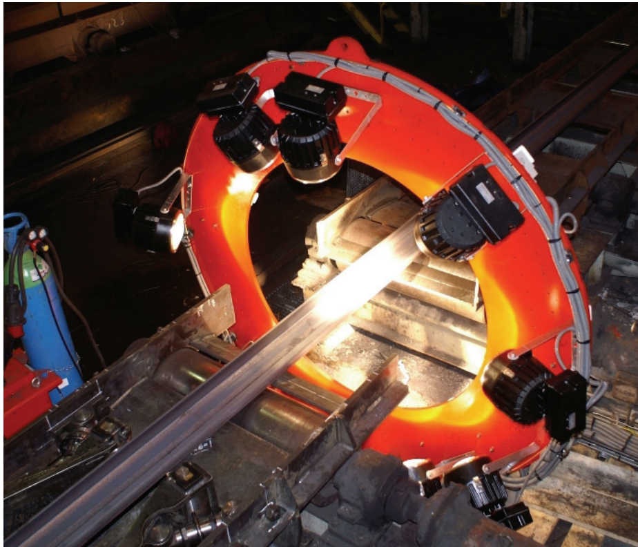
The inspection ring (lamp side) during commissioning
