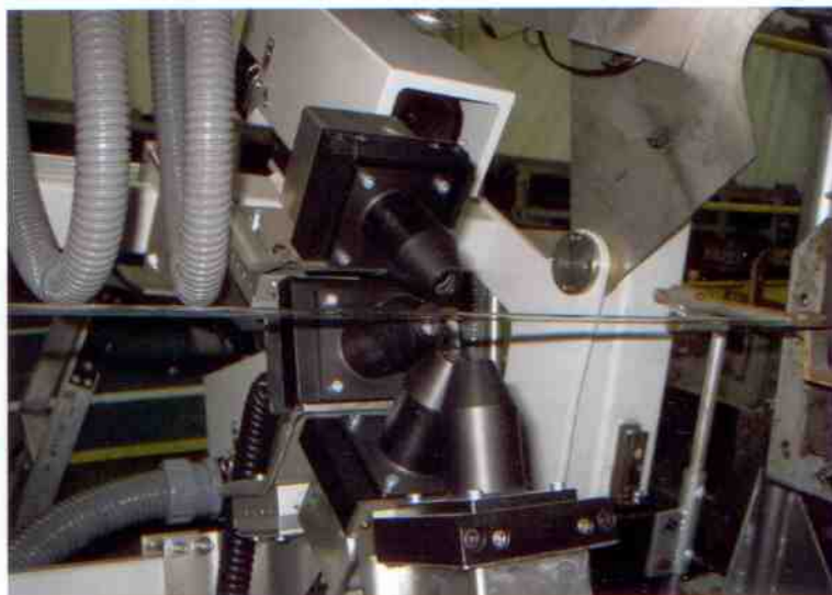
Close up of the quadruple optical system.
